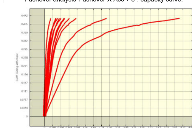
Pushover analysis"Pushover-Y Acc + e": capacity curve.
