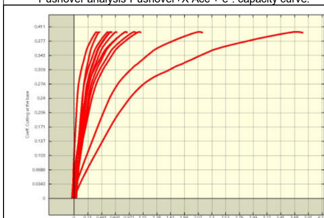
Pushover analysis"Pushover+Y Acc + e": capacity curve.
