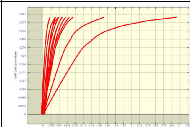
Pushover analysis"Pushover-Y Acc - e": capacity curve.
