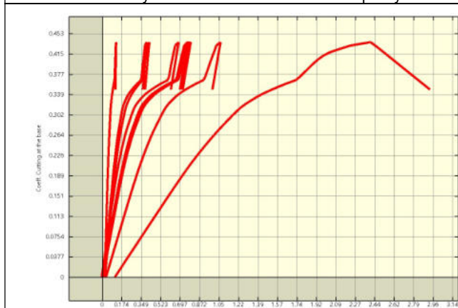
Pushover analysis"Pushover+X Acc + e": capacity curve.
