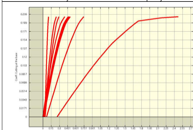
Pushover analysis"Pushover+X Acc": capacity curve.
