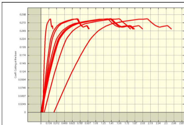
Pushover analysis"Pushover+X Massa - e": capacity curve.
