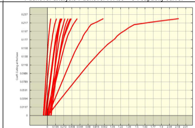
Pushover analysis"Pushover-Y Acc + e": capacity curve.
