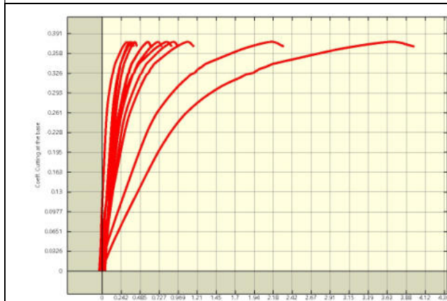
Pushover analysis"Pushover+Y Acc - e": capacity curve.
