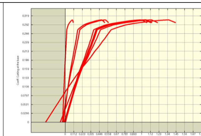
Pushover analysis"Pushover-X Massa - e": capacity curve.
