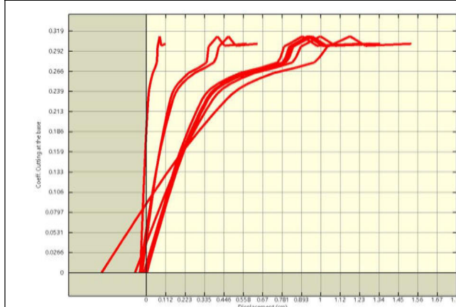
Pushover analysis"Pushover-X Massa": capacity curve.
