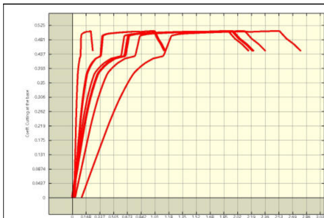
Pushover analysis"Pushover+X Massa - e": capacity curve.
